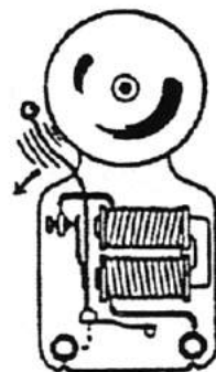
The clapper arm springs back.
