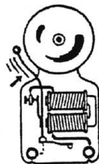
The flow of electricity again pulls the arm back.
