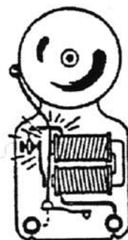
The clapper strikes the bell and breaks the current.
